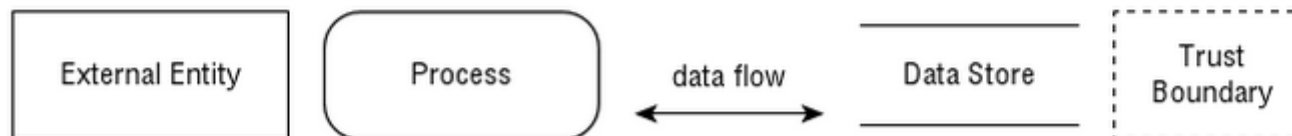
Figure 2-4: A modern DFD model (previously shown as Figure 2-1)
